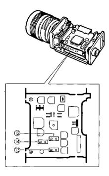
12. Gamma On/Off Switch ON COFF (SW 1)
